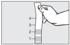
Dip the strip in your drinking water for approximately a second, then shake off any excess water. The result will be evident after about a minute. If the water is harder than 40°d/7.0 mmol/l, limescale will build up more rapidy than with soft water. Descaling will need to be carried out more regularly than stated to prevent limescale damage to the machine.
